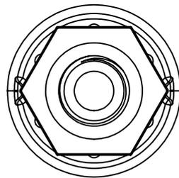
Hydrophobic and oleophobic breather
