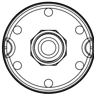
Hydrophobic and oleophobic breather
