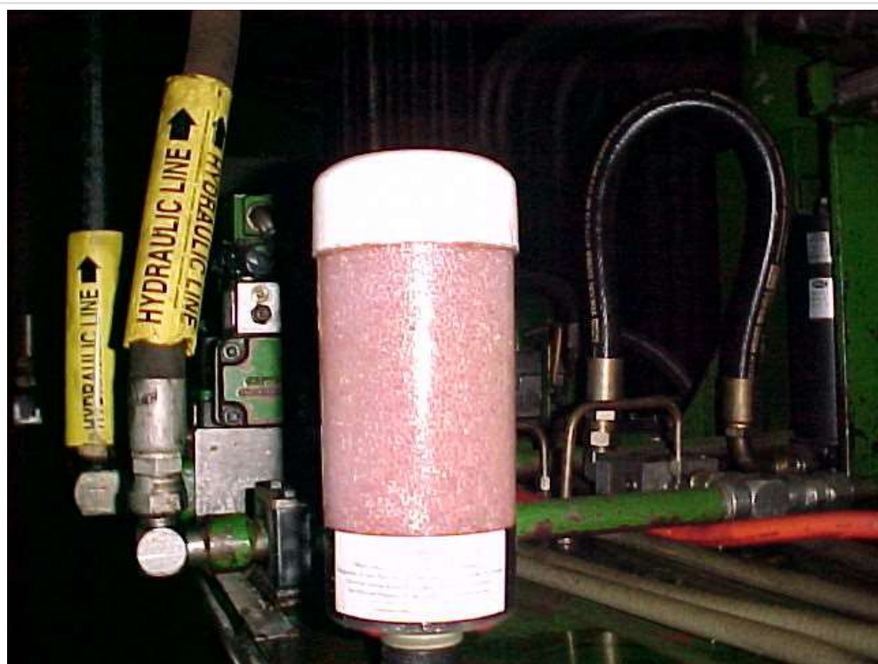
Hygroscopic Breather Saturated with Water
