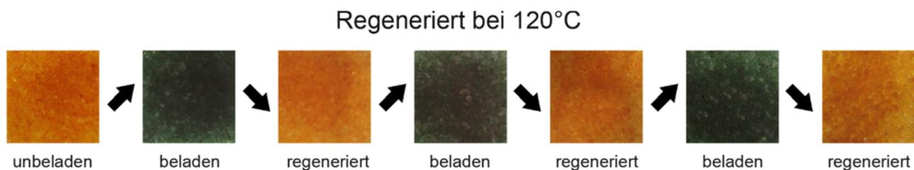
Abbildung 2: Color change by adsorption and regeneration.
