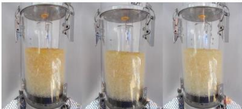
Figure: Photos show adsorbers at 10%, 20% and 30% total loading, silica gel 0.5kg (dry).
