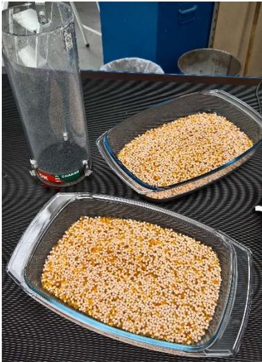
In this case the adsorbers were opened and tested regarding the general condition and loading state. The silica gel orange-colourless had adsorbed 555,7g water and was in a very good state.
