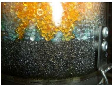
outflowing oil particles are bound and the cleaned air can be used for regeneration of the silica gel. This extends the service life of the silica gel and ensures better air drying.
