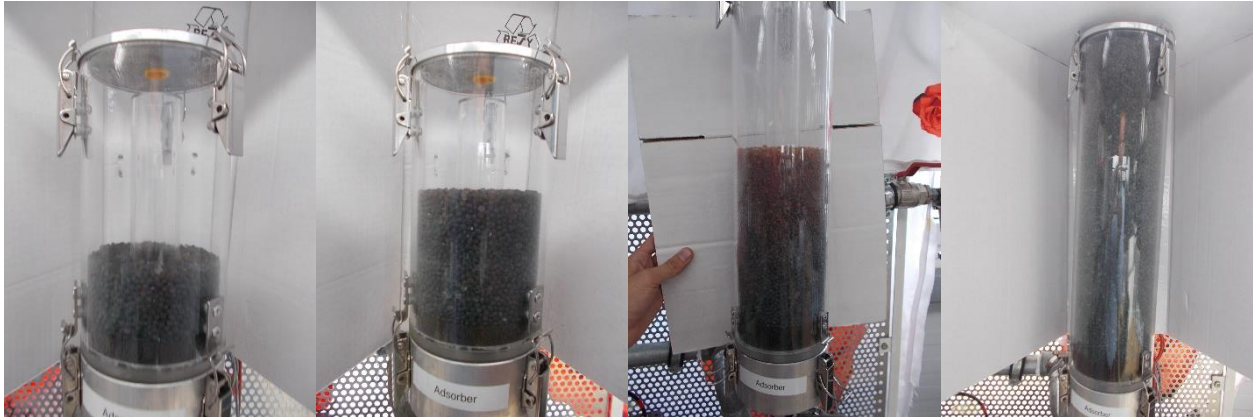
Figure: Tested amounts of silica gel (from left: 0.25kg, 0.5kg, 1kg, 2kg)
