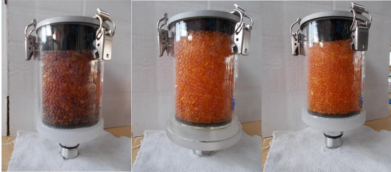
Figure: Adsorber tested **after 50 days** (left: holes, middle: membrane, right: valve).
