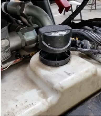
Picture 3: Hydraulic tank of a snow groomer.
