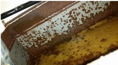
Picture 4: Water in hydraulic tank. Strongly aged hydraulic oil.
