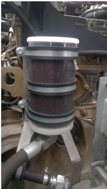
PA were installed. The air sucked into the tank is thus dehumidified to initially 2%rh (average 10%rh).
