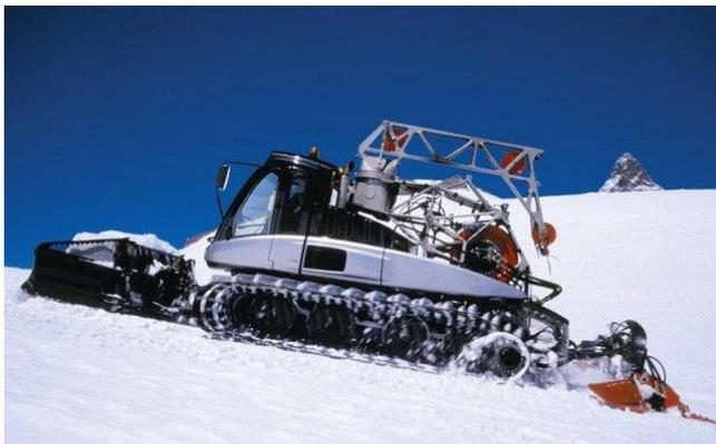
Picture 2: Snow groomer from Prinoth with attachments, operated hydraulically.
