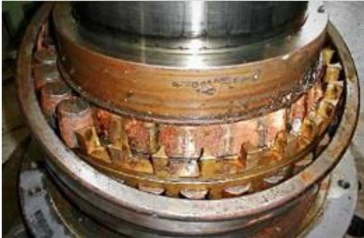
Due to the strong influence of temperature caused by the environment and the long downtimes, the formation of condensation is strongly favored. The intake air during cooling and the constant contact with the environment ensure that humidity flows into the transmission and liquefies on cooling.
