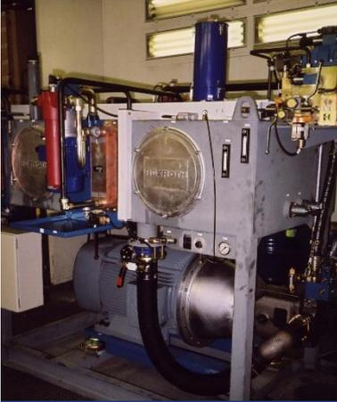
Hydraulic power units are used in oil circulation lubrication systems. These systems cool and lubricate bearings and gearboxes.
