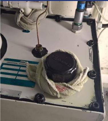
The operation of the oil is very warm and additionally quickly returned to the hydraulic tank so that it swirls in the tank and is present as an aerosol in the air.
