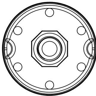
Hydrophobic and oleophobic breather
